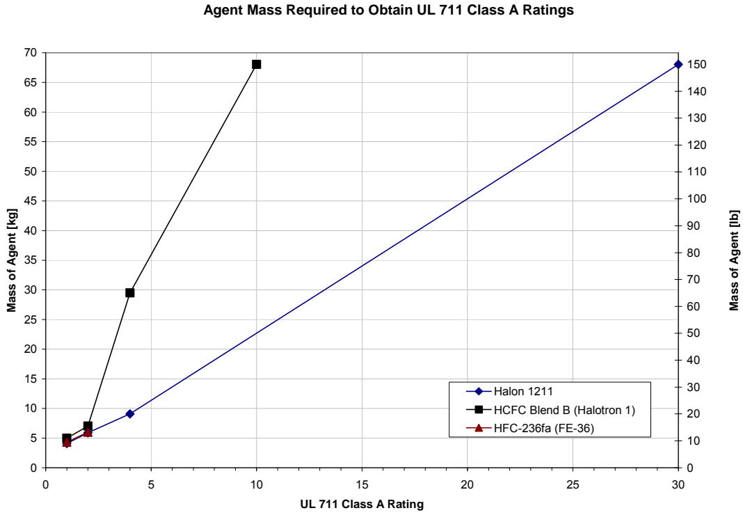
Figure 1 – Agent Mass Requirements to Obtain UL-711 Class A Extinguisher Ratings
